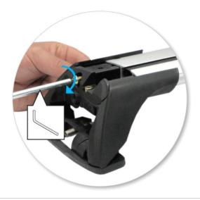
• Tighten adjusting screw to 5 Nm.
